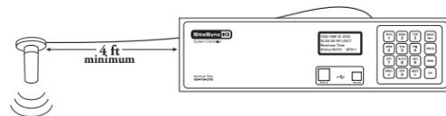
System controller located high & central with Ethernet drop for time reference
